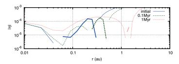
**Fig. A.1.** Time evolution of the absolute value of the scaling factor of pressure gradient force  $\eta$  for an MRI-inactive disk based on Suzuki et al. (2016). Thick lines correspond to the region where  $\eta$  is negative.
