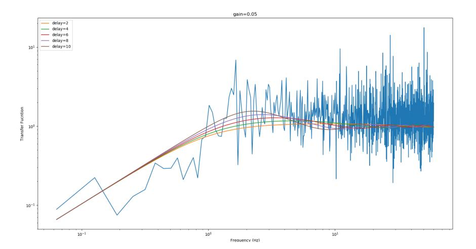
This plot (in blue) presents the first estimation of the transfer function of the GD close loop on the 15 baselines of the SPICA-FT testbed. It should be noted that the performance is not representative of what is expected as we are using a lab IR detector (exposure time 8ms) and a very old computer.
